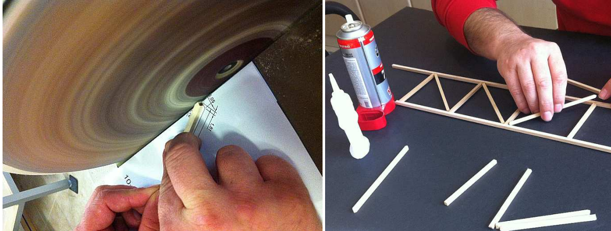
Figure 4: (a) Construction of a connection using model building equipment (b) Model assembly
