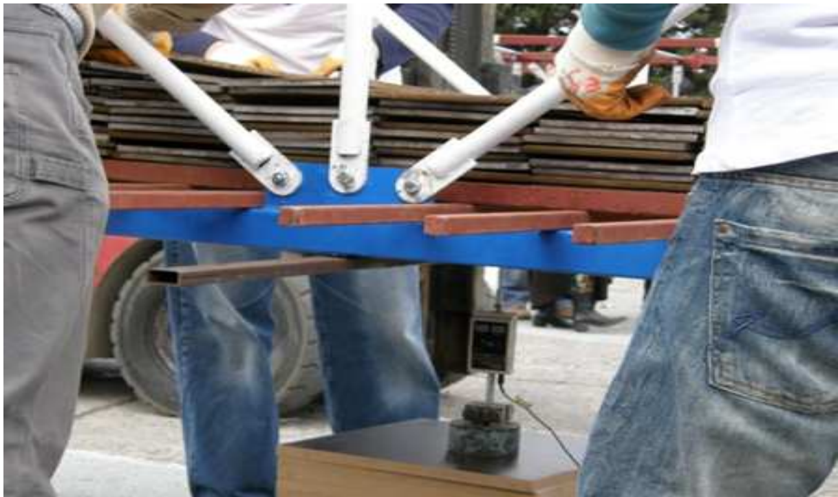
Figure 4: Application of the Vertical Loads to the Bridge.
